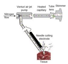
Beam me up: A novel mass spectrometric ionization technique based on rapid evaporation of biological tissues (see picture) can be used to analyze vital tissues during surgical intervention as well as for processed tissue specimens. A tissue identification system based on principal-component analysis was developed. The method differentiates malignant tumor cells from the surrounding healthy tissue.
