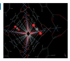
The diffusion mechanism of CO₂ in the highly flexible metal—organic framework MIL-53(Cr) (see picture), which undergoes a structural transition between large-and narrow-pore forms, was explored by a combination of quasi-elastic neutron scattering measurements and molecular dynamics simulations. Normal one-dimensional diffusion in the large-pore form and single-file one-dimensional diffusion in the narrow-pore form were evidenced.
