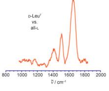
Differential IR spectra of gas-phase proteins at room temperature can be obtained by a combination of IR multiphoton dissociation (IRMPD) and FT ion cyclotron resonance mass spectrometry. This new approach yields unique spectra for all-L and singly D-substituted isomers of the protein Trp-cage (see depicted differential spectrum) and thus avoids possible unfolding of proteins during IR irradiation that can affect conventional IRMPD measurements.
