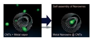
Filling the tube: Ultrathin metal nanowires with diameters of single atoms (ca. 1.7 nm) were synthesized in high yield by using a nanofilling reaction using the nanospace of carbon nanotubes (CNTs).
