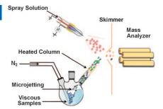
Sticky subject: An N<sub>2</sub> stream forms bubbles inside bulk viscous liquids, which create an aerosol sample through a microjetting mechanism (see picture). This aerosol is then analyzed by extractive electrospray ionization (EESI) mass spectrometry (MS). EESI-MS reveals the molecular composition of complex liquids and the kinetics of ongoing processes occurring in the highly viscous liquids without any sample pretreatment.
